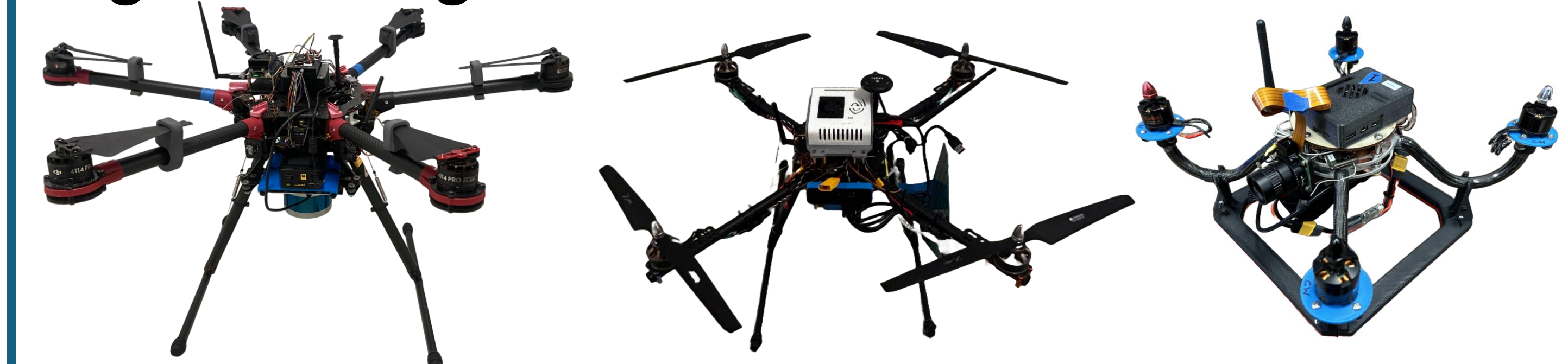
Figure 4: From left to right: the Heavy Drone Class, able to map the area and complete visual tasks; the Medium Drone Class, able to complete visual, thermal, and radio tasks; and the Light Drone Class, able to complete visual tasks. All drones are able to serve as mesh nodes.
