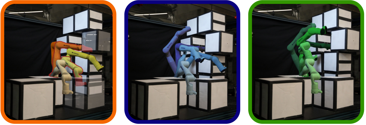
Figure 3.1: This chapter introduces BLAZE, a Phase 1 - Phase 2 Affine Geometric Heat Flow (AGHF) framework, to rapidly solve optimal control problems while respecting robot constraints and avoiding obstacles. It begins with an initial trajectory (shown in orange with the color gradient illustrating the evolution in time starting from darkest and going to lightest) that may violate constraints (e.g., the second and fourth pose of the arm are in collision with the boxes and outlined in red ). If the initial trajectory is infeasible, BLAZE enters Phase 1, where it evolves the trajectory into a trajectory that satisfies all constraints (e.g., in the blue trajectory, the Kinova arm has been moved out of collision with the boxes). Once the trajectory satisfies all constraints, Phase 2 begins, optimizing the motion to minimize a user-specified cost function while maintaining feasibility (optimized trajectory shown green ). BLAZE optimizes the trajectory to reach a target configuration while avoiding the obstacles while considering the full dynamical model of the arm. Note that optimal control (including Phase 1 and Phase 2) for this 14 dimensional state space model is completed within 3s while satisfying input, state, and collision avoidance constraints.
