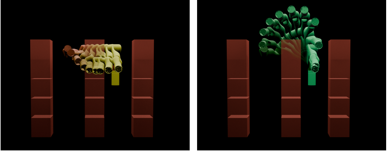
Figure 3.4: This figure shows a visualization of BLAZE’s solution for one of the 2-second horizon task-based scenarios (scenario 3). In each subfigure, the color gradient illustrates the evolution in time where the start configuration is in the darkest shade and the end configuration in the lightest. The initial trajectory for the scenario is shown in the top image in yellow and collides with the obstacles along the path. The proposed algorithm is able to push this initial guess out of collision and generate the optimal collision-free solution shown in green in 3.73s for this scenario, whereas the other comparison methods cannot find a solution within the allotted time for this scenario.
