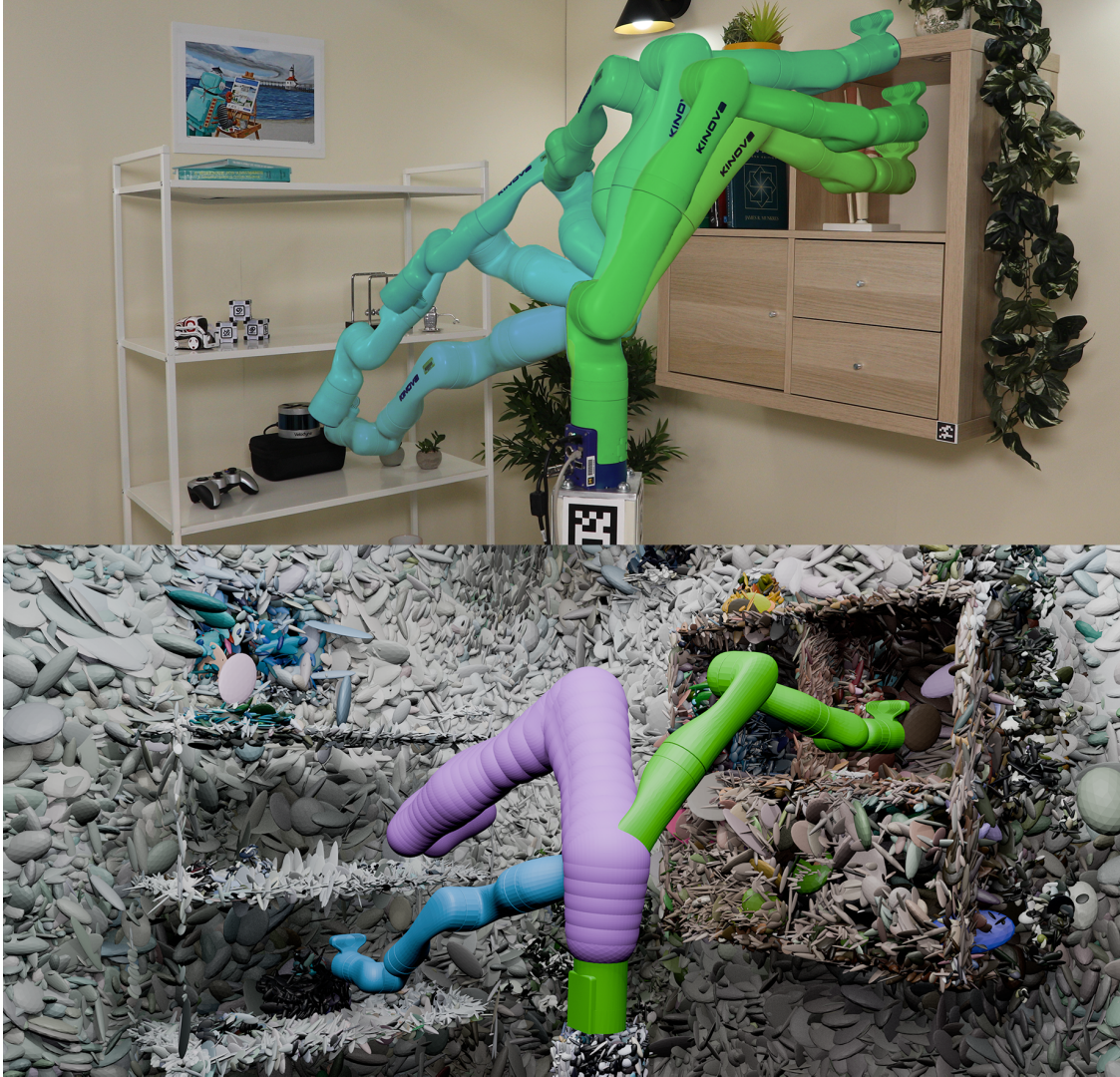
Figure 5.1: SPLANNING constructs risk-aware trajectories in a Gaussian Splatting map in real-time. The top image shows a real-world scene that a 7DOF serial manipulator must plan through, starting at the blue configuration (left) and ending at the green configuration (right). The scene is represented as a normalized 3D Gaussian Splat. Then, in real-time, SPLANNING solves an optimization problem that constrains the probability that the robot’s forward occupancy (bottom center, purple ) collides with the scene.
