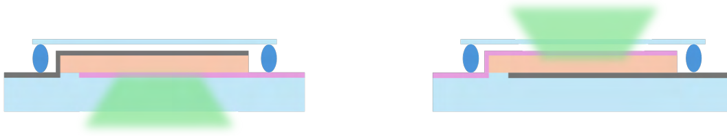
Figure 1.3: Schematic of bottom-up and top-down devices. Side view of bottom-up ( left ) and top-down ( right ) devices. The organic areas are indicated in orange. Transparent and opaque contacts are indicated by the pink and gray areas, respectively. The substrate/encapsulation glass and epoxy seal are indicated by light and dark blue, respectively.
