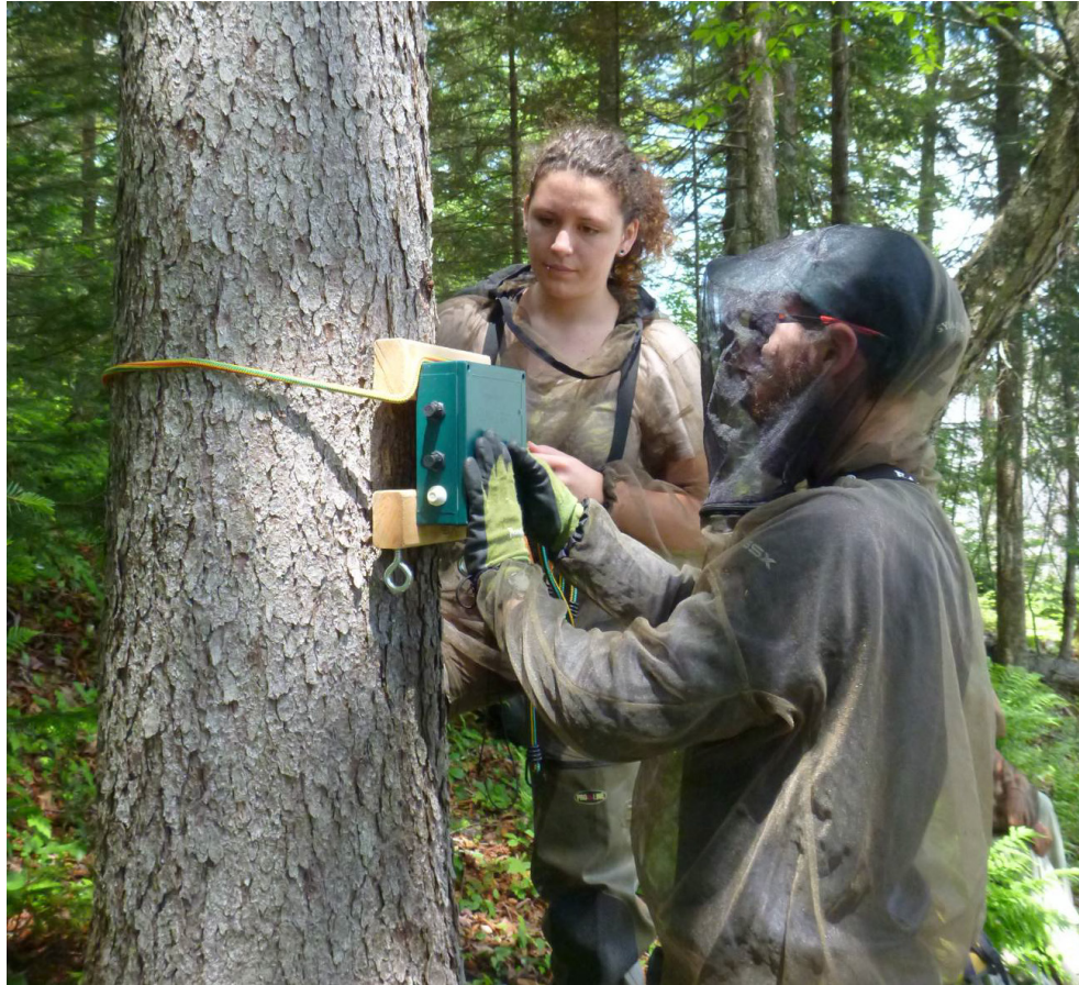
Fig. 3. Students at SUNY ESF's Adirondack Ecological Center install an automated recording system to survey the biological soundscape. Photograph by Stacy A. McNulty.
