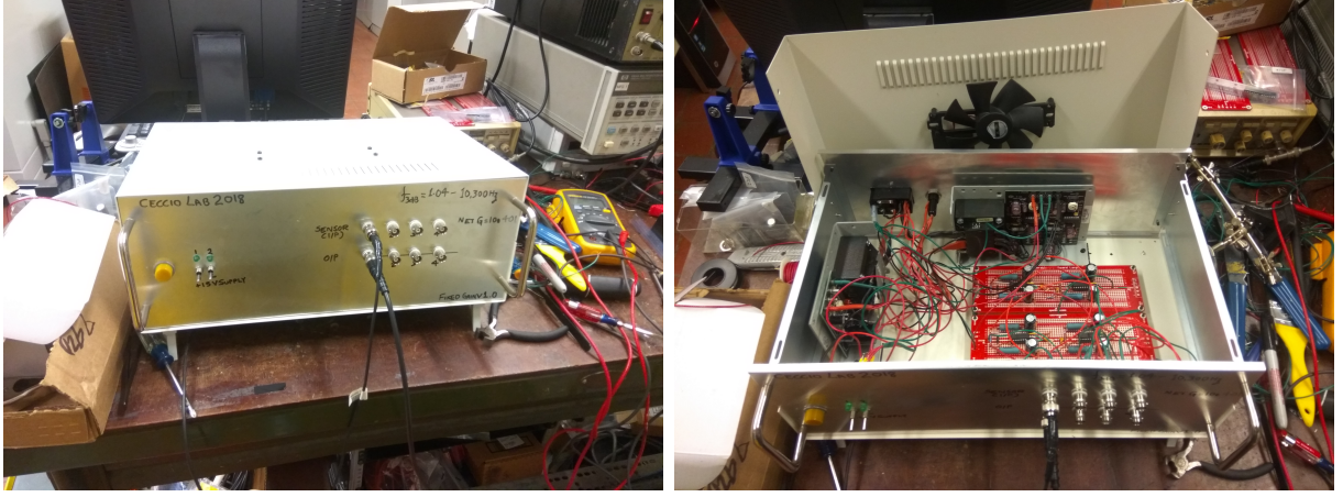
Figure A.2: Assembled charge amplifier box with grounded instrument casing and BNC connections.
