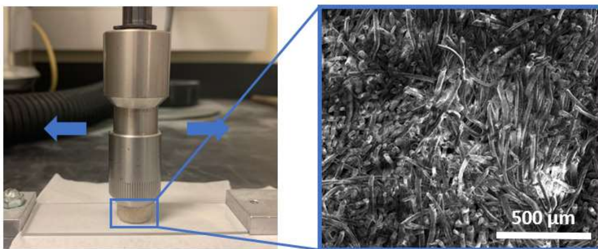
Figure 48: Linear Tabor abrasion setup for antifog coated polycarbonate and the microstructure of the CS-5 felt tip abrasion tip.
