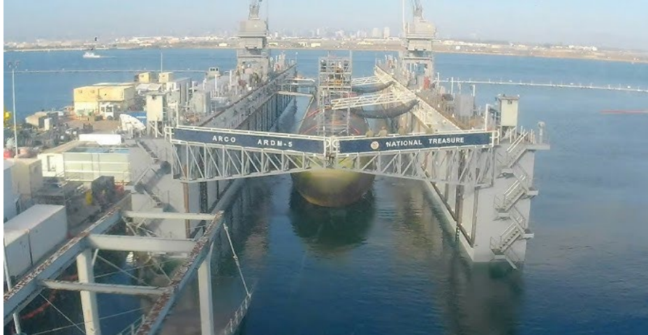
Figure 2.2.2 US Navy Submarine USS Scranton onboard a partially submerged floating dry dock, San Diego, CA. See link for timelapse of the submersion and floating process. ( https://www.youtube.com/watch?app=desktop&v=YX8h-bfrAr4 )
