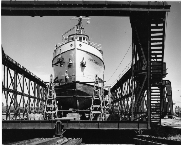
16-A-3 (4) D Marine Railway - showing bow view of Tuna Clipper "SUN DAWN". Industrial Division, Cristobal, Canal Zone. 4/20/54 Figure 1.2.4 Vessel, Sun Dawn, on a marine railway, 1954.
