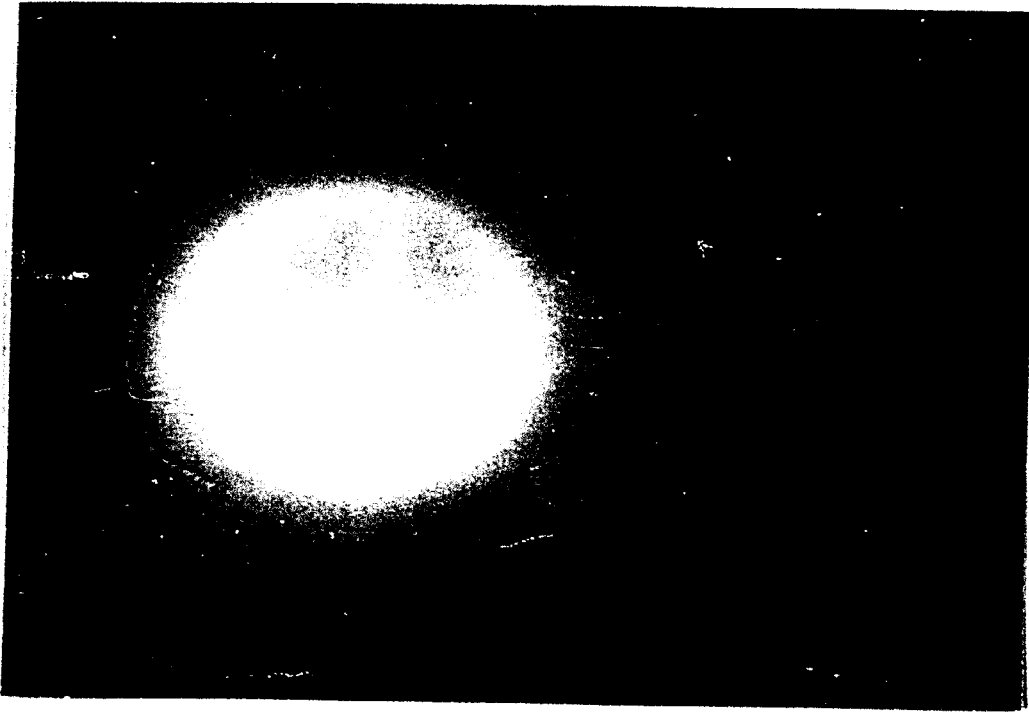
Figure 5. Photograph of X-Ray Beam Taken at Entrance Port to Experimental Area.
