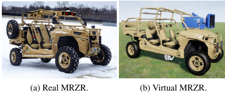
Figure 2.3: A real (left) and virtual (right) Polaris MRZR vehicle. Left: An MRZR vehicle used by the Automotive Research Center at the University of Michigan. Right: A rendering of an MRZR as used in the UE4 simulations.
