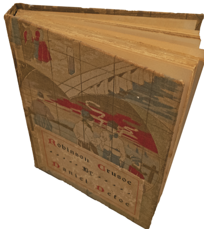
Fig. 13. Square-back publishers' binding, printed cloth, 1899. The binding has a square back, but the stiff inlay is not the full thickness of the boards. The book block is wire-stitched and backed. Aikin, Lucy. Robinson Crusoe: His Life and Strange, Surprising Adventures by Daniel Defoe, in Words of One Syllable . Philadelphia: Henry Altemus Co., 1899. Courtesy University of Michigan Library (Special Collections Research Center).
