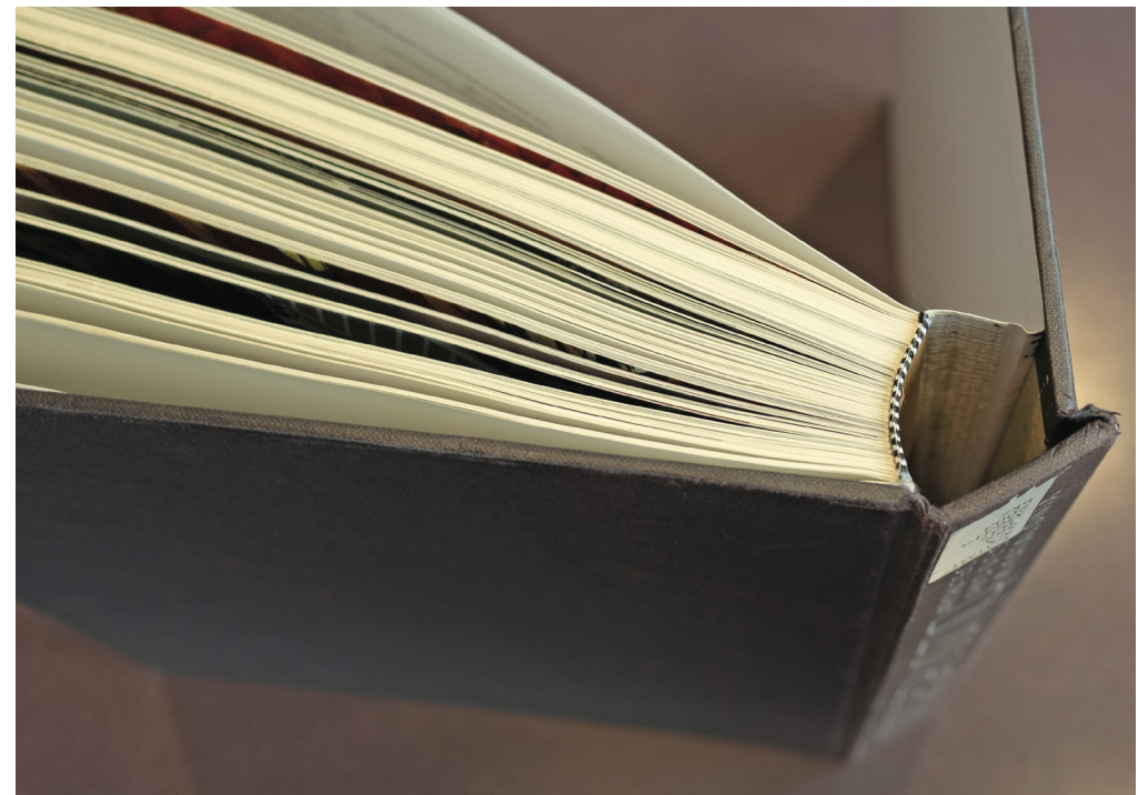
Fig. 6. Typical damage to a square-back, stiff-spine case after use: the endsheet along the hinge is levered off the board.
